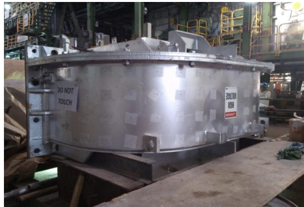
Image 12: High Voltage electrically charged Inductor
